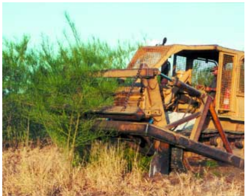
Mechanical control with an Ellrott front-mounted bladeplough. Photo: John McKenzie
