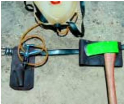
Stem injection can be conducted on foot using a 5 L backpack, injector gun and small axe. Photo: Ian Holloway, QPWS
