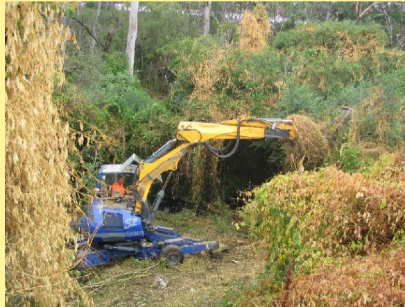
The low resilience sites were treated using “tritter” machinery, which have been developed to clear vegetation economically and safely in forestry situations...
