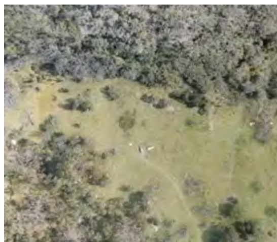
This photo stitch example shows an MS ICE (image composite editor) stitch of 145 individual photos taken at 80 metres above ground level on a prearranged flight plan. (supplied by author).
